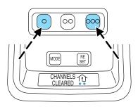
**Do not** repeat step one to program additional hand-held transmitters to the remaining two HomeLink® buttons. This will erase previously programmed hand-held transmitter signals into HomeLink®.
